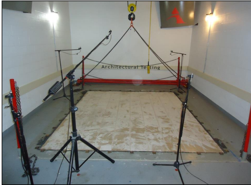
Source Room View of Test Specimen Installation
